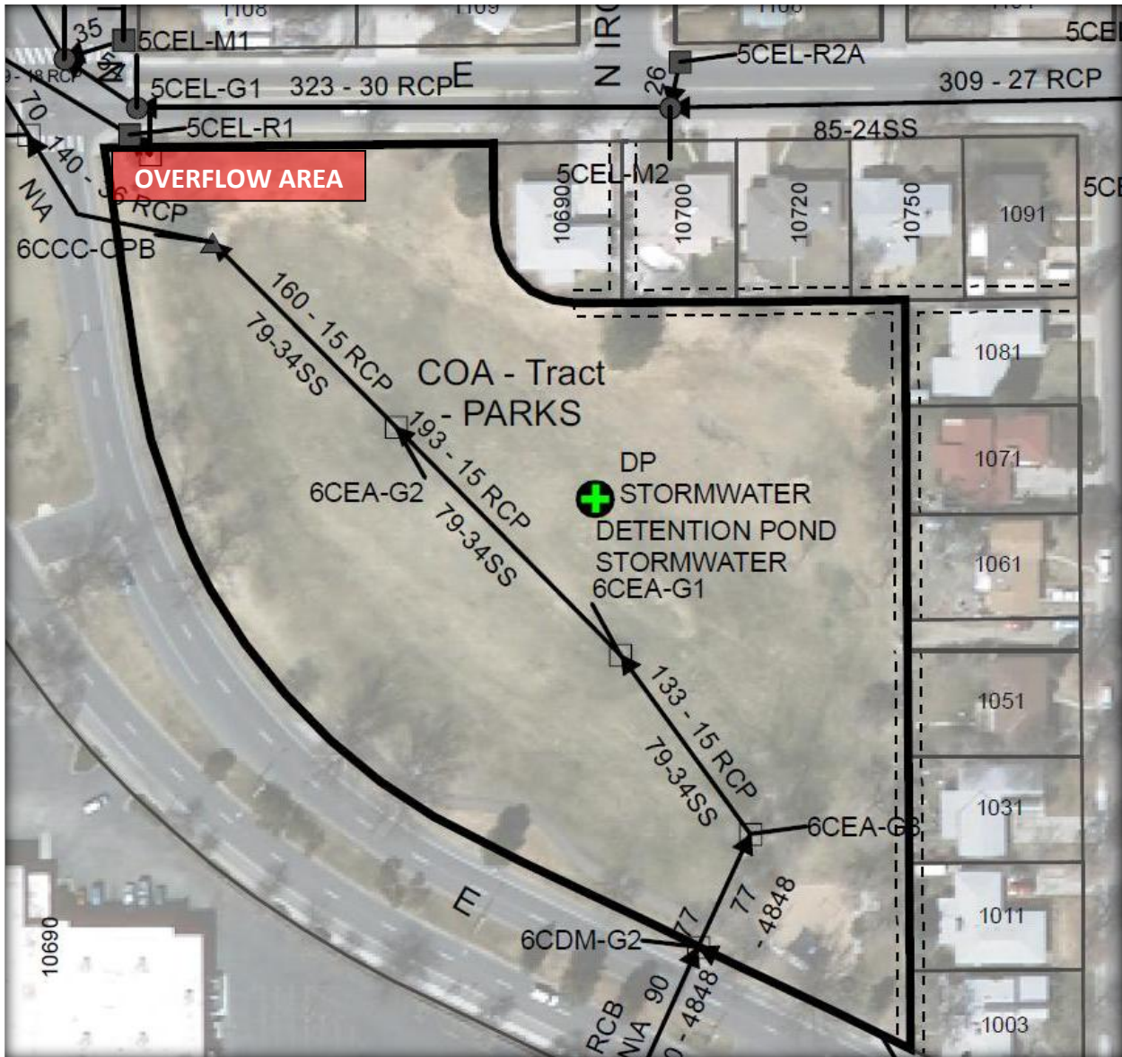
Aerial Photo and map of 11 th and Del Mar Pkwy. Notice the locations of the inflow grate, the two low-flow grates and the outflow structure.
