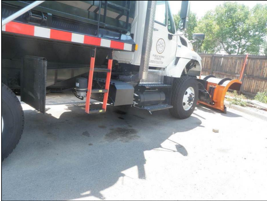
Photograph 17. View facing southwest at petroleum product staining on the impervious surface underneath a stored vehicle. Note the lack of spill response BMP implementation.
